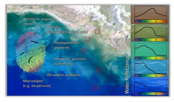
**Figure 1**. The 5 panels (right) display the spectrum of light corresponding to the ocean color shown. The shape of the color intensity changes across the spectrum, providing a unique fingerprint imparted by the materials in the water.
