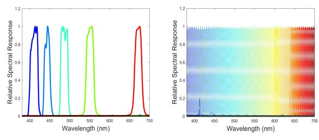
**Figure 2**. (Left) The relative spectral response of the Visible Infrared Imaging Radiometer Suite (VIIRS) sensor compared to that of PACE (right). Narrower bandwidth and more bands are what constitute the "hyperspectral" nature of spectrometers.
